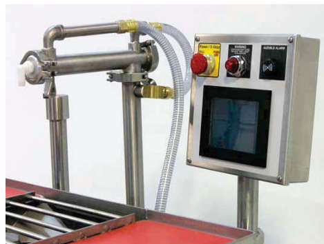
Water-jacketed depositing nozzle & pipe
