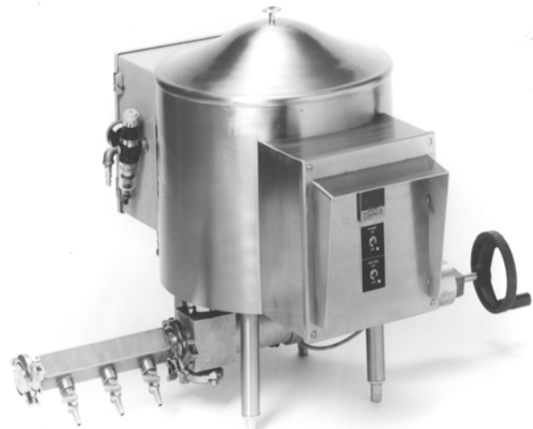
50 lb Table Top Tank with depositing pump & 3 nozzles
