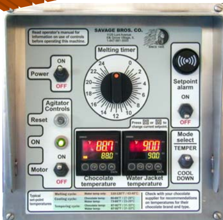
Control cover features 24 hour melt timer and two digital temperature controllers for accurate water & chocolate control
