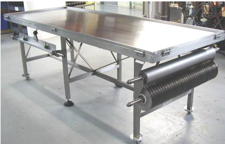
Drum Sizer, Product Leveler and Roller Cutter shown on Savage water-jacketed Cooling Table, with handy saddles to store processing tools.
